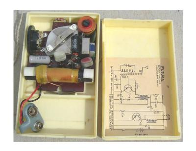
1950s transistor radio could be taken apart to see how they work
