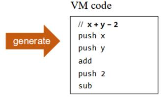
When executed during runtime, the generated code ends up leaving the value of the expression at the stack's top
